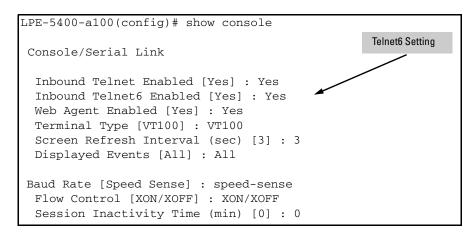
Figure 5-5. Show Console Output Showing Default Console Configuration
